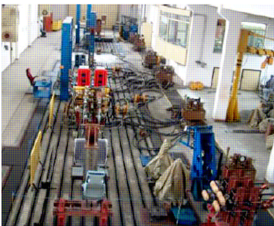
Fig. 1. Hydropuls installation for testing in simulated and accelerated regime
