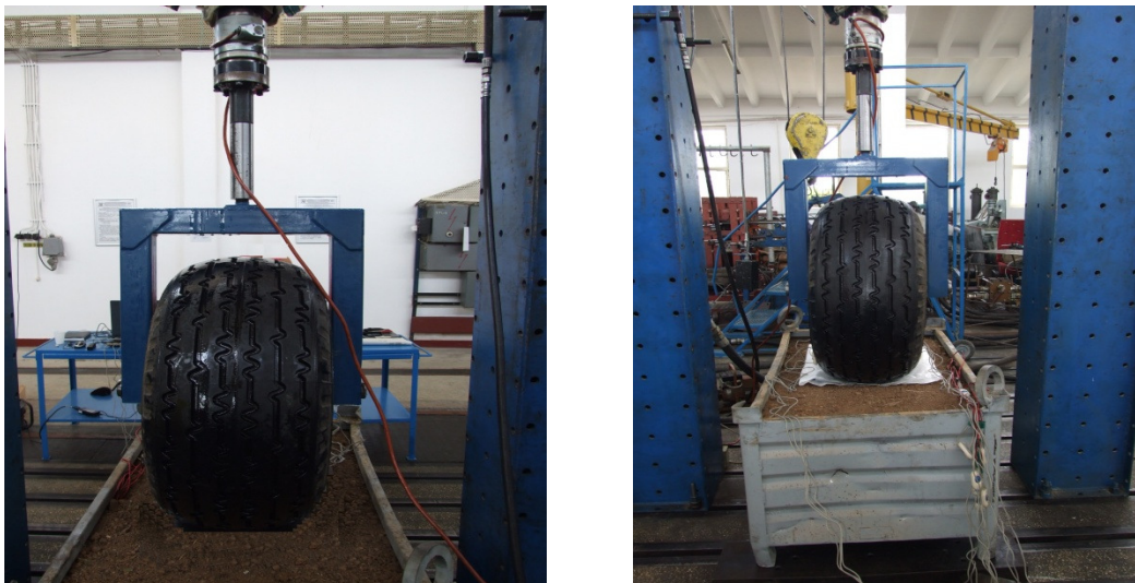
Fig. 4. Simulation of static compression pressure for tire of corn harvester
